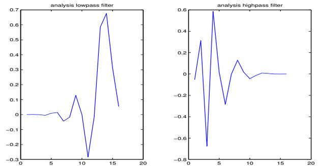
Fig. 3. Daubechies analysis filters. The left figure shows the low pass filter and the right figure shows high pass filter. The filters are designed for the number of coefficients to be 16. X axis indicates the coefficient number, while the Y axis shows the value for that coefficient number. The filter is normalized so that sum of all the filter coefficients is equal to  $\sqrt{2}$ .
