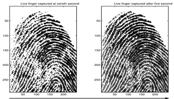
Fig. 1. Live fingerprint images captured as a time sequence. The left figure is captured immediately after placement of finger on the scanner (zeroth second), while the right is captured after five seconds. Perspiration is observed as time progresses.
