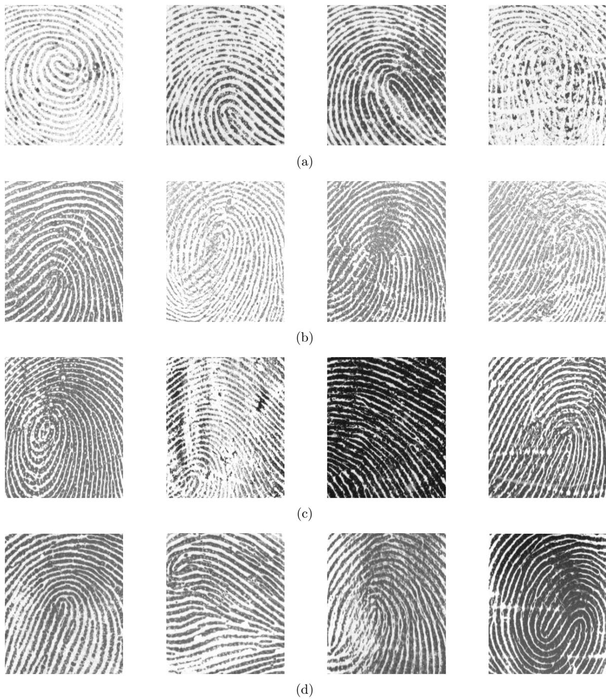
Figure 3: Example of live and non-live fingerprints captured by Identix DFR2100 scanner: (a) live fingerprint; (b) Play-Doh spoof sample; (c) Gelatin spoof sample; (d) Silicone spoof sample.
