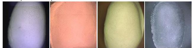
Fig. 2. Photos of spoof fingers made from various materials (left to right: latex caulk, latex paint, Play-Doh, and silicon).
