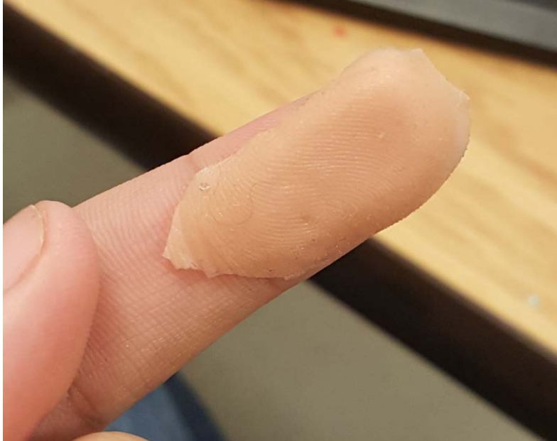
Figure 2. Biometric spoofs can be created which is difficult to spot, e.g. a skin colored, thin fingerprint spoof can be glued to a user's actual finger.
