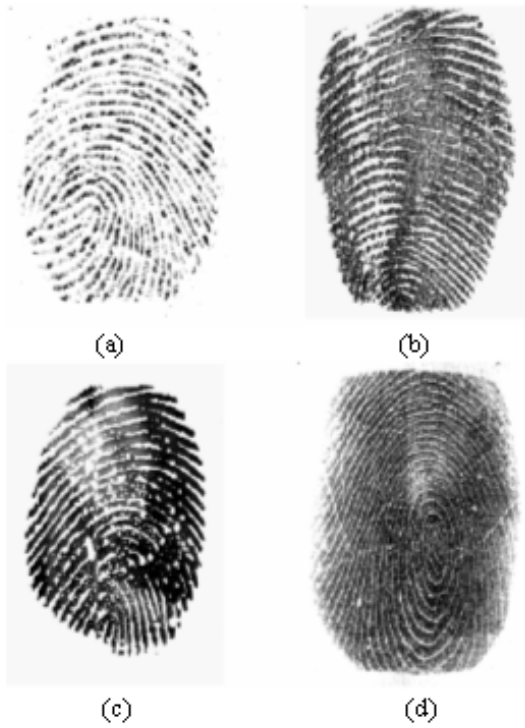
Fig. 1. Example of live and non-live fingerprints captured by Capacitive DC scanner: (a) live finger; (b) spoof finger made from Play-Doh; (c) spoof finger made from gelatin; (d) cadaver finger
