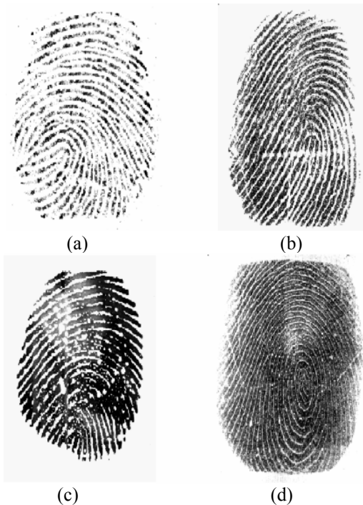
Figure 1: Example of live and non-live fingerprints captured by Capacitive DC scanner: (a) live finger; (b) spoof finger made from Play-Doh; (c) spoof finger made from gelatin; (d) cadaver finger
