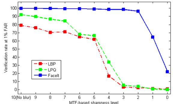
Figure 6: Verification rates at 1% FAR for three face recognition algorithms on Q-FIRE with MTF-based sharpness levels
