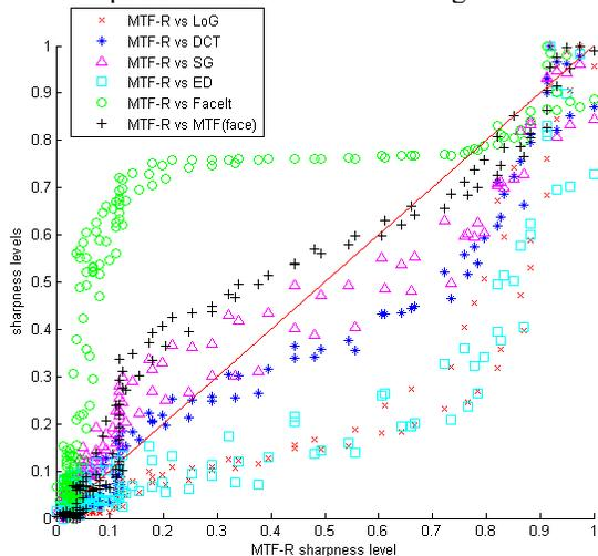
Figure 3: Example comparisons of normalized blur measurements for one subject: MTF-R versus LoG, DCT, SG, ED, FaceIt and MTF of the face region. 0 presents the lowest sharpness level and 1 presents the sharpest (no blur) level.
