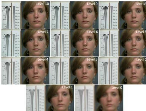
Figure 1: Example frames of real out-of-focus blur from Q-FIRE dataset with standard optical chart on the side of face at 5ft
