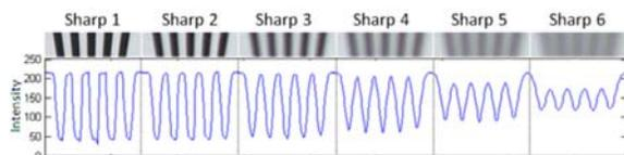
Figure 2: Example of intensities of number 2 region from the standard optical chart showing 6 different sharpness levels (from sharpest to blurry) within one video sequence
