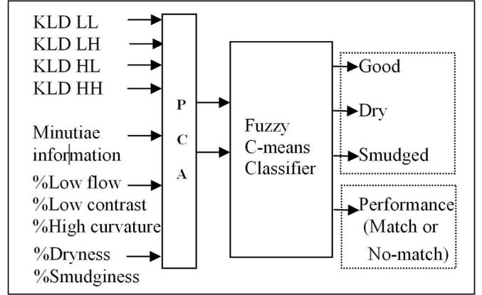
Fig. 3. Classification scheme with different features as input for predicting a match or a no match.
