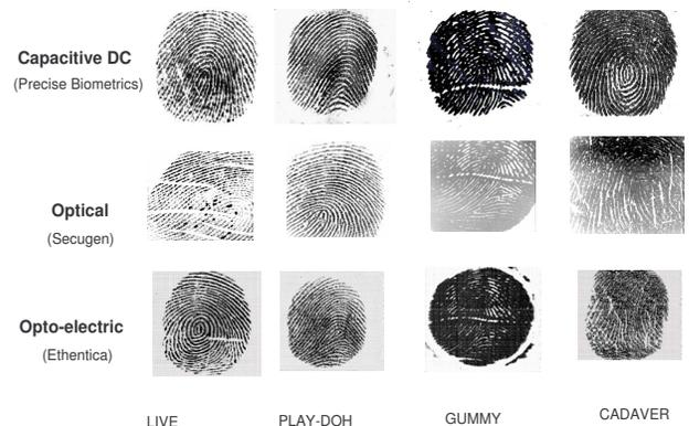
**Fig. 1.** Fingerprint image samples for live, play-doh spoof, gummy and cadaver are shown in columns, for three different fingerprint sensing technologies, namely capacitive DC, optical and opto-electrical, shown in rows.
