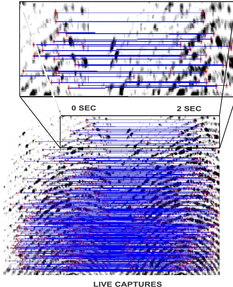
Figure 2. Live fingerprint captures at 0sec and after 2sec are shown with the key points linked.
