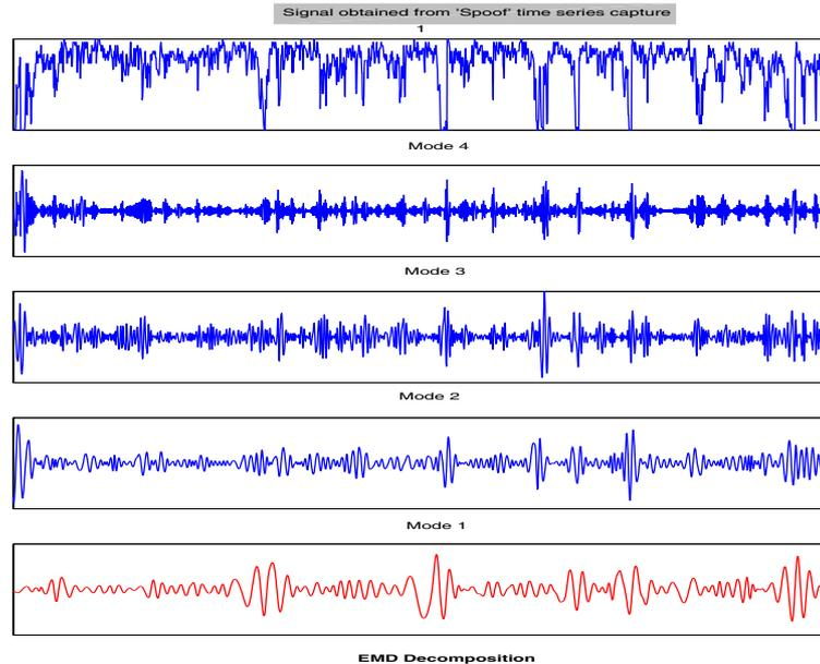
Figure 5. EMD Decomposition for the spoof fingerprint signal.
