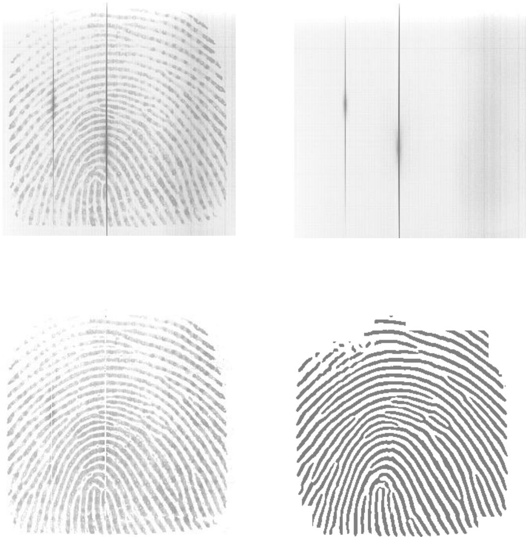
**Figure 5** Original scan (top left), blank scan (top right) and scan after noise and defects removed (bottom left), and binary image (bottom right).
