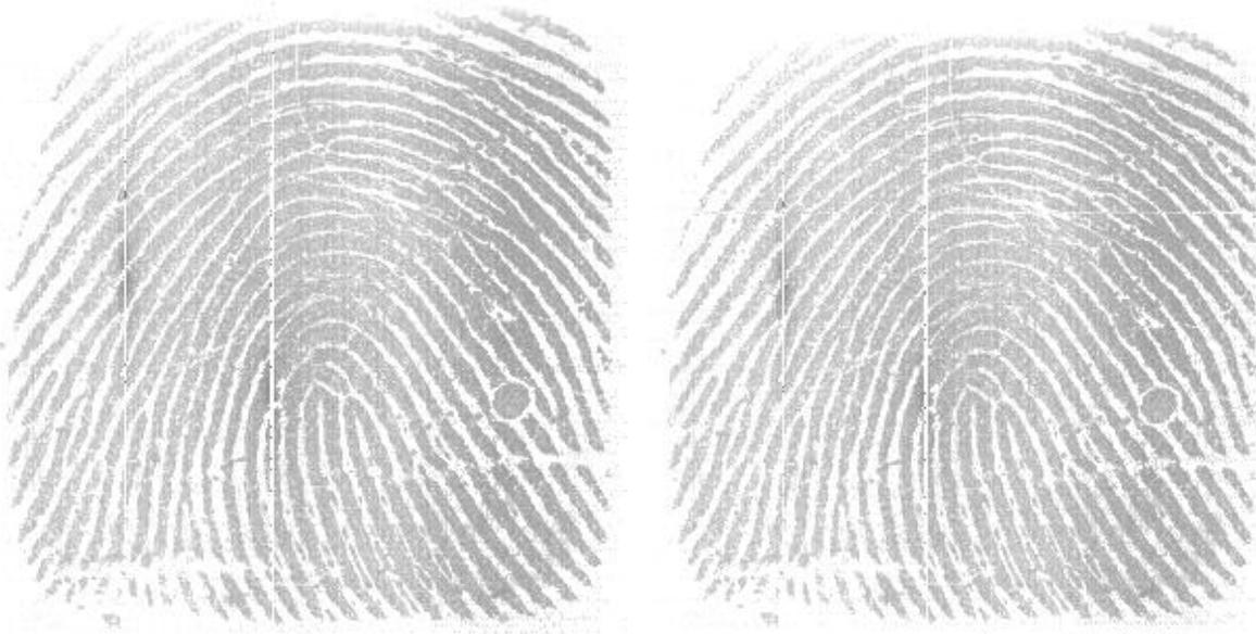
**Figure 4** The first (left) and last (right) scan of a spoof fingerprint.
