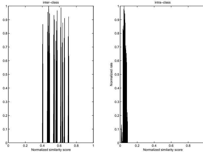
**Fig. 4.** Results of characterization of perspiration pattern. Similarity scores for inter and intra-class patterns. The similarity score is normalized. The intra class can be seen very similar, and inter class can be seen distributed around 0.6, and hence very much random.
