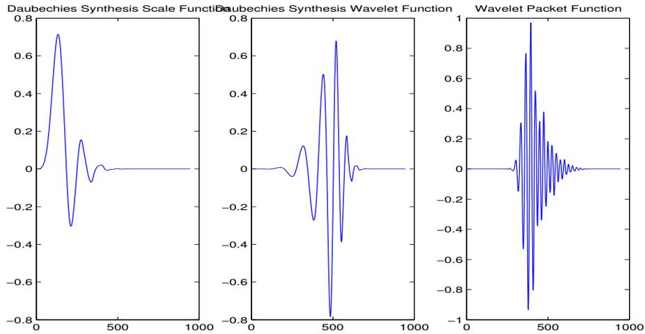
**Figure 3.** Left figure indicates Daubechies scale function ( $\phi$ ), middle figure indicates Daubechies wavelet function ( $\psi$ ), and right figure shows the wavelet packet function. For all the figures the number of iterations are selected to be 5.
