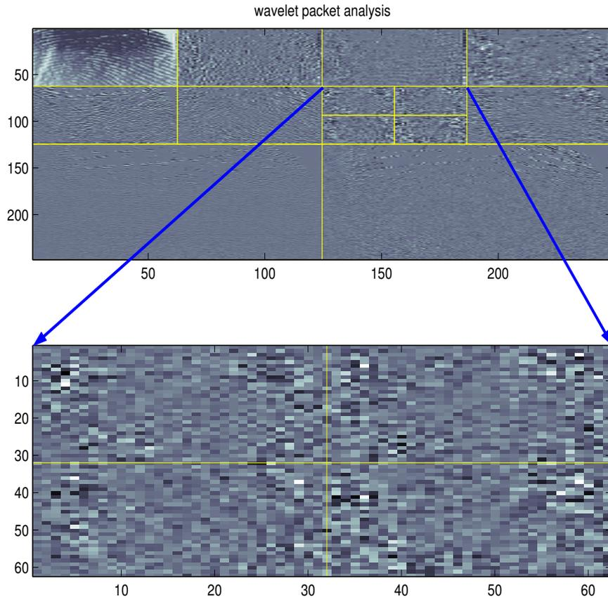
**Figure 5.** Wavelet packet transform. The scale selected is 3, and all the sub-bands are marked. Only high pass scale 3 sub-bands are retained for further analysis. Those are shown separately.
