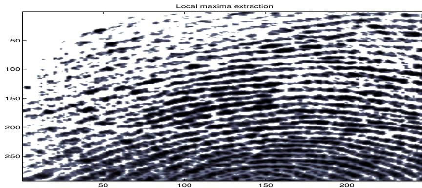
**Figure 4.** Maxima energy extraction. The figure shows a sample fingerprint image after retaining the most significant 10000 coefficients. This image is produced after making these coefficients undergo inverse transform.
