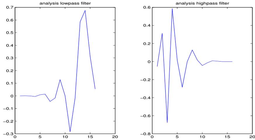
**Figure 2.** Daubechies analysis filters. The left figure shows low pass filter and the right figure shows high pass filter. The filters are designed for number of coefficients to be 16. X axis indicates the coefficient number, while the Y axis shows the value for that coefficient number. The filter is normalized so that sum of all the filter coefficients is equal to  $\sqrt{2}$ .
