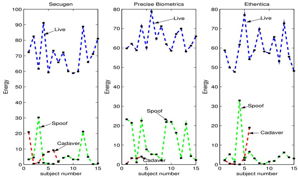
**Figure 7.** Training data set results. The graphs are for optical, capacitive DC, and opto-electrical scanners respectively, from left to right. Clear separation among energy distributions of ‘live’, and ‘not live’ fingers is obtained.
