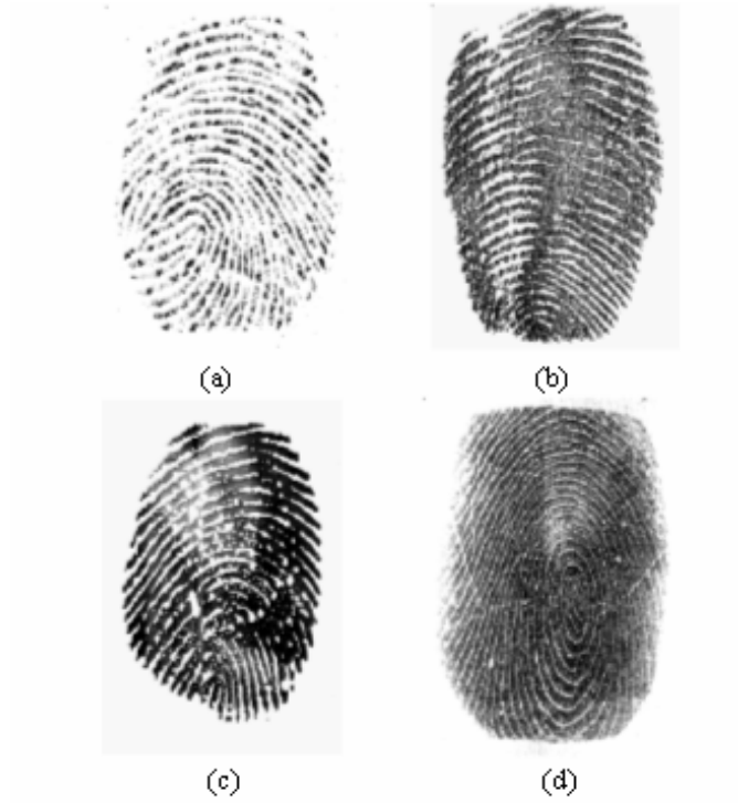
Fig. 1. Example of live and non-live fingerprints captured by Capacitive DC scanner: (a) live finger; (b) spoof finger made from Play-Doh; (c) spoof finger made from gelatin; (d) cadaver finger
