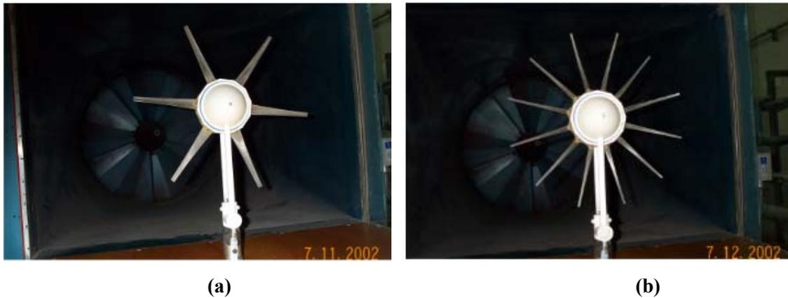
**Figure 1. Wind Tunnel Turbine Geometries**
