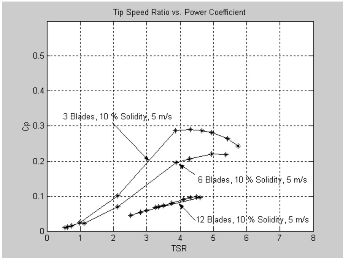
**Figure 3. Effect of Blade Number on Aerodynamic Performance**
