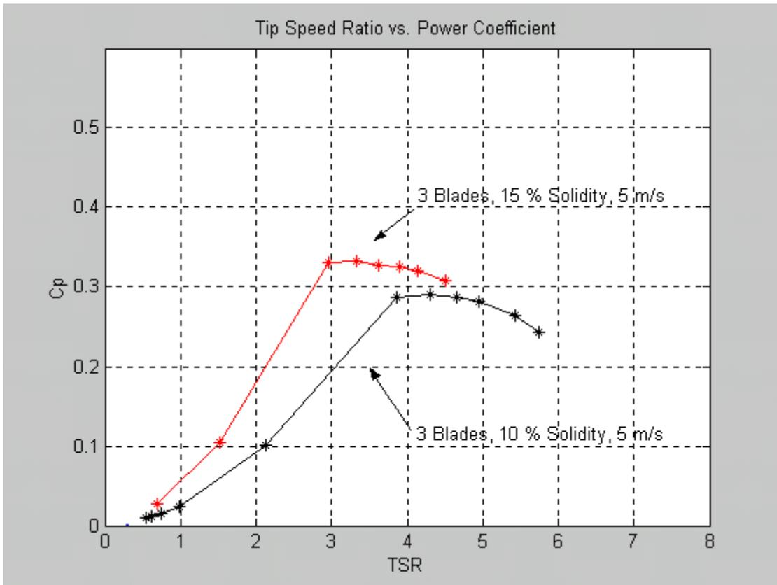
**Figure 2. Effect of Solidity on Aerodynamic Performance**
