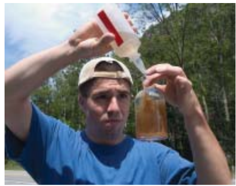
Joseph Osso Jr. processes a water sample used to measure dissolved oxygen as part of a study to examine the effects of road salt on Adirondack lakes.
